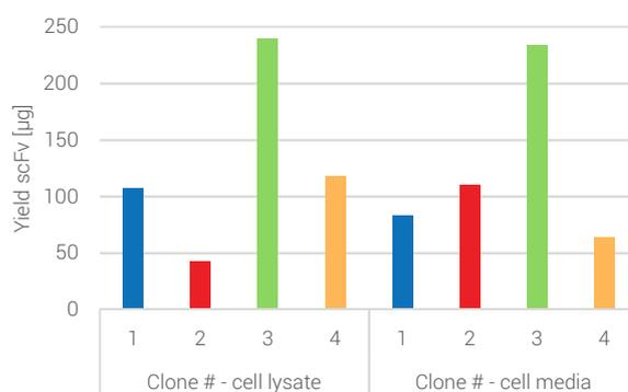
Fig 1. Yield of scFv from either 10 ml clarified bacterial cell lysate using a KingFisher Flex robot or directly from 500 ml cell culture media using the LOABeads MagSep50 and 500 magnetic separators, and a magnetic microtube rack.
